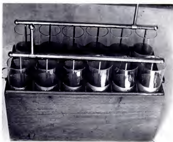
FIGURE 19. Battery of Leyden Jars. The box is labeled "JCM" [James Clerk Maxwell], "Electrical Apparatus belonging to Henry Cavendish." Photograph by the authors. Devonshire Collection, Chatsworth. Reproduced by permission of the Chatsworth Settlement Trustees.
